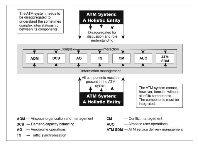
Figure 2-1. The seven ATM concept components
