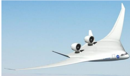
Blended Wing Body (NASA/Boeing)
