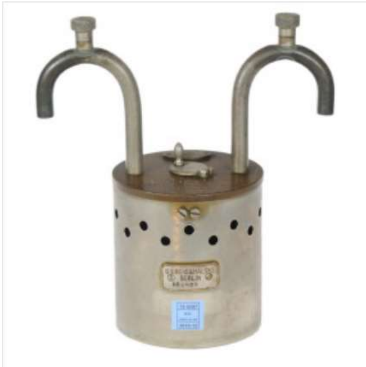
Normalwiderstand, 1 Ohm \pm 0,001\% , Siemens & Halske, 1897
