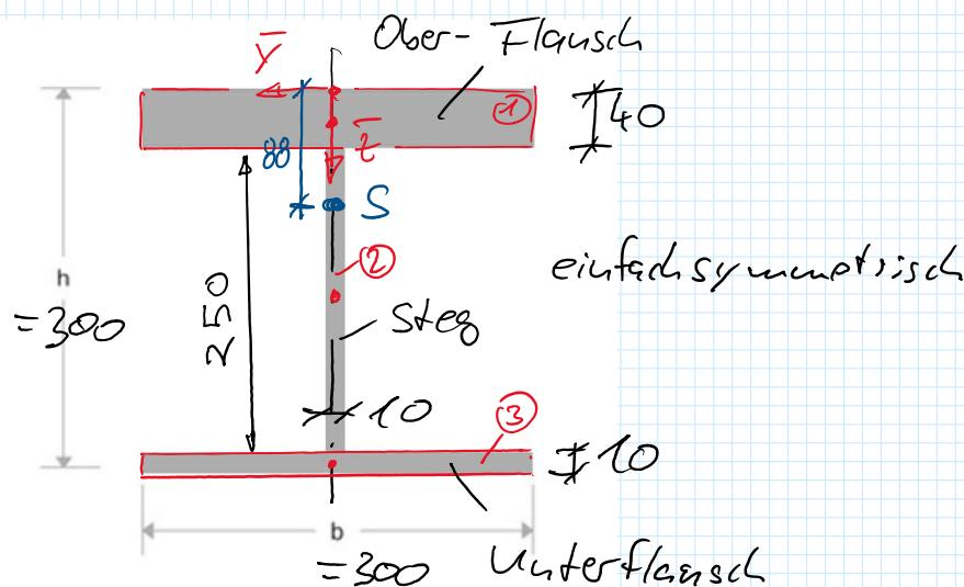
$$\bar{y}_s = \frac{\sum_{i=1}^n A_i \cdot \bar{y}_i}{\sum_{i=1}^n A_i} = 0 \quad \text{wg. Sym.}$$
