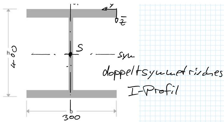
$$\bar{y}_s = \frac{\sum_{i=1}^n A_i \cdot \bar{y}_i}{\sum_{i=1}^n A_i} = \frac{300}{2} = 150 \quad \left. \begin{array}{l} \text{aus} \\ \text{Symmetrie} \end{array} \right\}$$
