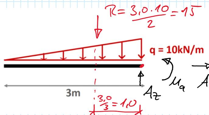
$$\begin{aligned}\sum F_x &= 0 \Rightarrow A_x = 0 \\ \sum F_z &= R - A_z \Rightarrow A_z = R = 15 \text{ kN} \\ \sum M_a &= 0 = 15 \text{ kN} \cdot 1,0 \text{ m} + M_q \\ \Rightarrow M_q &= -15 \text{ kNm}\end{aligned}$$
