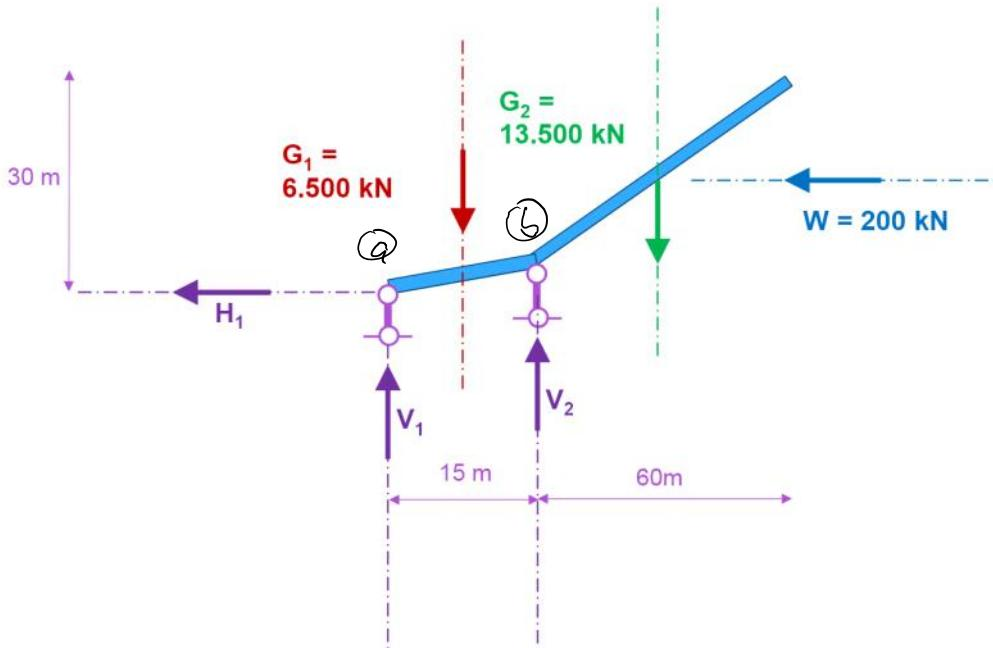
$$\sum F_{x_i} = 0 = -H_1 - 200 \text{ kN} \Rightarrow H_1 = -200 \text{ kN}$$
