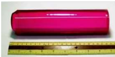
Large Czochralski Ruby Laser Rod Section for Faceting
