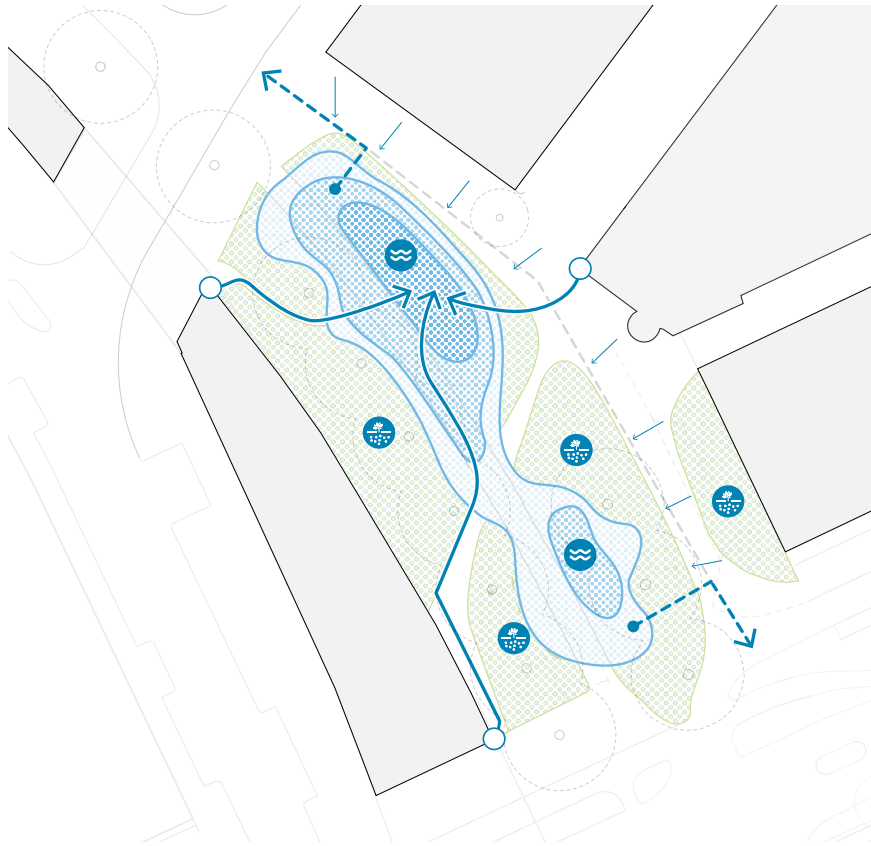
The deepest part attracts the water flow from the surroundings
